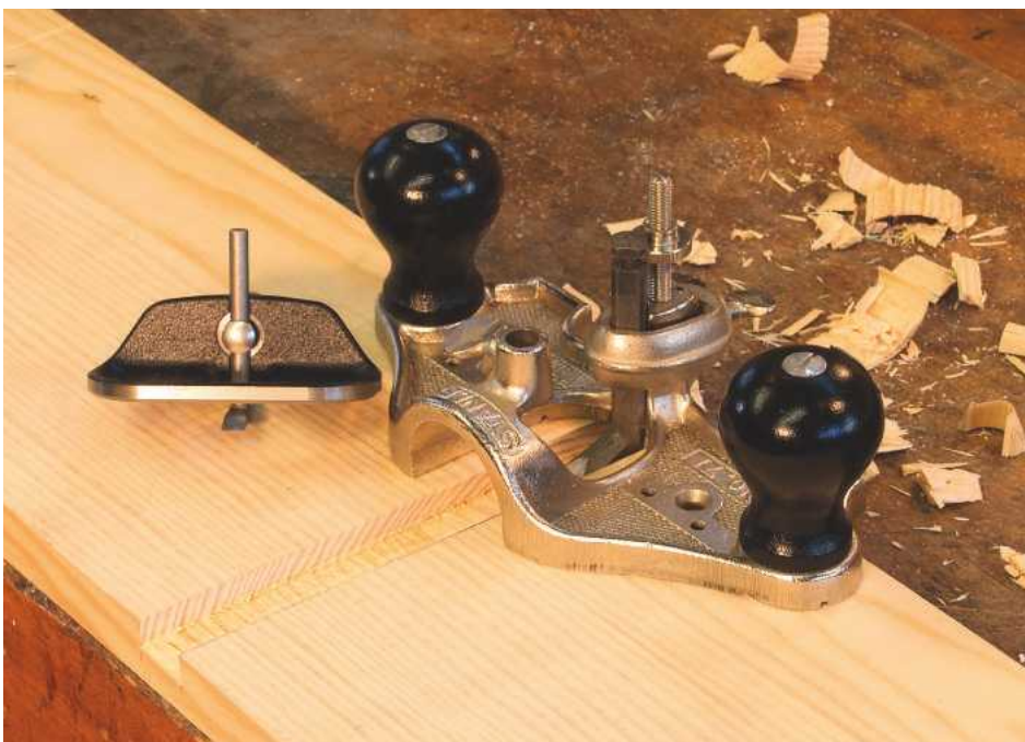
▲ Pic.5 Hand routers come in two sizes and are very useful
